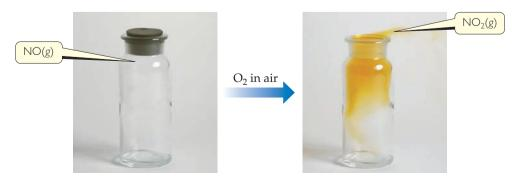
▲ Figure 22.24 Formation of NO<sub>2</sub>(g) as NO(g) combines with O<sub>2</sub>(g) in the air.
