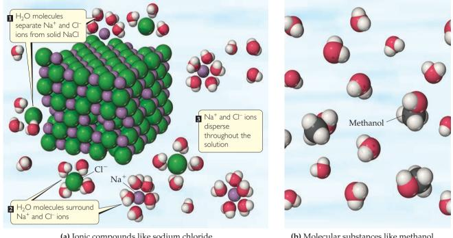
(a) Ionic compounds like sodium chloride, NaCl, form ions when they dissolve.
