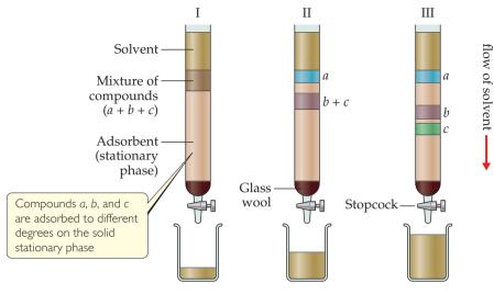
▲ Figure 1.14 Separation of three substances using column chromatography.
