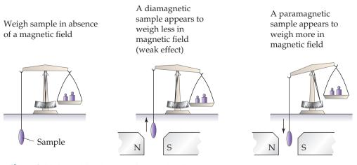
Figure 9.44 Determining the magnetic properties of a sample.
