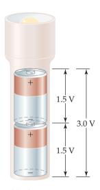
▲ Figure 20.18 Combining batteries. When batteries are connected in series, as in most flashlights, the total voltage is the sum of the individual voltages.
