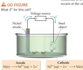
▲ Figure 20.29 Electrolytic cell with an active metal electrode. Nickel dissolves from the anode to form  $Ni^{2+}(aq)$ . At the cathode  $Ni^{2+}(aq)$  is reduced and forms a nickel "plate" on the steel cathode.
