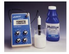
▲ Figure 16.7 A digital pH meter. The device is a millivoltmeter, and the electrodes immersed in a solution produce a voltage that depends on the pH of the solution.
