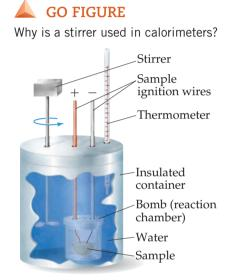
▲ Figure 5.18 Bomb calorimeter.
