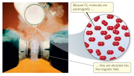
▲ Figure 9.45 Paramagnetism of 0<sub>2</sub>. When liquid oxygen is poured through a magnet, it "sticks" to the poles.
