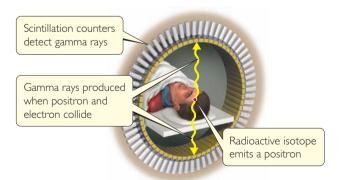
▲ Figure 21.10 Schematic representation of a positron emission tomography (PET) scanner.
