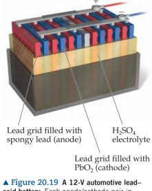
acid battery. Each anode/cathode pair in this schematic cutaway produces a voltage of about 2 V. Six pairs of electrodes are connected in series, producing 12 V.
