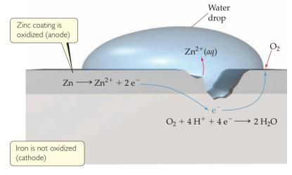
▲ Figure 20.26 Cathodic protection of iron in contact with zinc. The standard reduction potentials are  $E_{\text{red. Fe}^{2+}}^{\circ} = -0.440 \text{ V}$ ,  $E_{\text{red. Zn}^{2+}}^{\circ} = -0.763 \text{ V}$ , making the zinc more readily oxidized.
