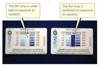
▲ Figure 21.8 Badge dosimeters monitor the extent to which the individual has been exposed to high-energy radiation. The radiation dose is determined from the extent of darkening of the film in the dosimeter.
