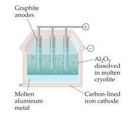
▲ Figure 20.32 The Hall–Héroult process. Because molten aluminum is denser than the mixture of cryolite ( $Na_3AIF_6$ ) and  $AI_2O_3$ , the metal collects at the bottom of the cell.
