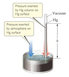
▲ Figure 10.2 A mercury barometer.
