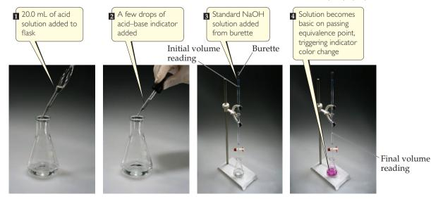
▲ Figure 4.18 Procedure for titrating an acid against a standard solution of NaOH. The acid–base indicator, phenolphthalein, is colorless in acidic solution but takes on a pink color in basic solution.
