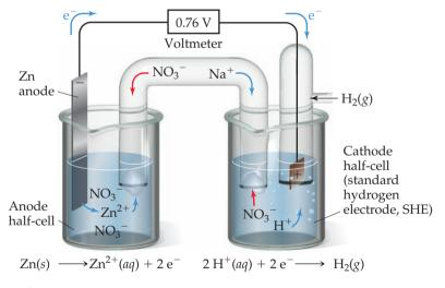
▲ Figure 20.9 A voltaic cell using a standard hydrogen electrode (SHE). The anode half-cell is Zn metal in a  $Zn(NO_3)_2(aq)$  solution, and the cathode half-cell is the SHE in a  $HNO_3(aq)$  solution.
