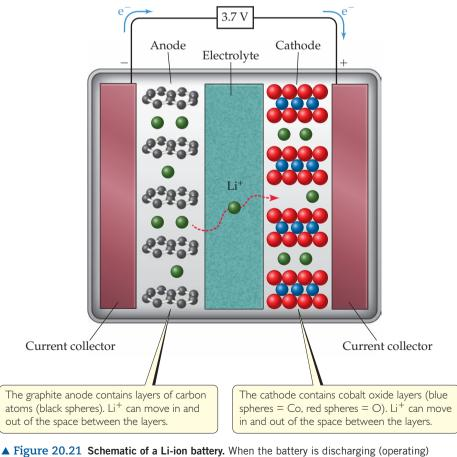
Li<sup>+</sup> ions move out of the anode and migrate through the electrolyte where they enter the spaces between the cobalt oxide layers, reducing the cobalt ions. To recharge the battery, electrical energy is used to drive the Li<sup>+</sup> back to the anode, oxidizing the cobalt ions in the cathode.
