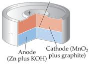
▲ Figure 20.20 Cutaway view of a miniature alkaline battery.
