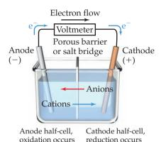
▲ Figure 20.6 Summary of reactions occurring in a voltaic cell. The half-cells can be separated by either a porous glass disc (as in Figure 20.4) or by a salt bridge (as in
