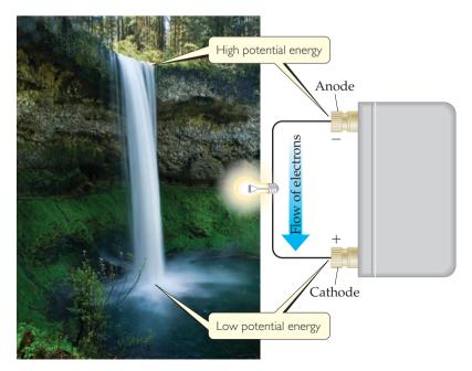
▲ Figure 20.7 Water analogy for electron flow.
