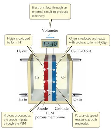
▲ Figure 20.24 A hydrogen-PEM fuel cell. The proton-exchange membrane (PEM) allows  $H^+$  ions generated by  $H_2$  oxidation at the anode to migrate to the cathode, where  $H_2O$  is formed.
