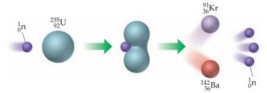
▲ Figure 21.13 Uranium-235 fission. This is just one of many fission patterns. In this reaction,  $3.5 \times 10^{-11}$  J of energy is released per <sup>235</sup>U nucleus that is split.
