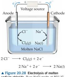
sodium chloride. Pure NaCl melts at 801 °C.
