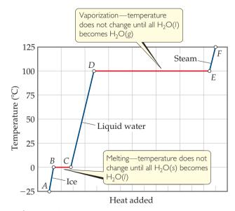
▲ Figure 11.22 Heating curve for water. Changes that occur when 1.00 mol of H<sub>2</sub>O is heated from H<sub>2</sub>O(s) at -25 °C to H<sub>2</sub>O(g) at 125 °C at a constant pressure of 1 atm. Even though heat is being added continuously, the system temperature does not change during the two phase changes (red lines).
