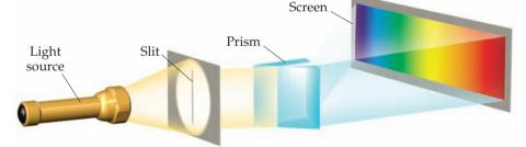
▲ Figure 6.9 Creating a spectrum. A continuous visible spectrum is produced when a narrow beam of white light is passed through a prism. The white light could be sunlight or light from an incandescent lamp.
