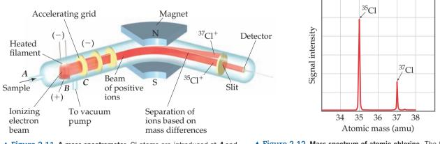
▲ Figure 2.11 A mass spectrometer. CI atoms are introduced at *A* and are ionized to form  $CI^+$  ions, which are then directed through a magnetic field. The paths of the ions of the two CI isotopes diverge as they pass through the field.
