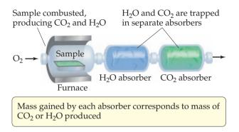
▲ Figure 3.14 Apparatus for combustion analysis.
