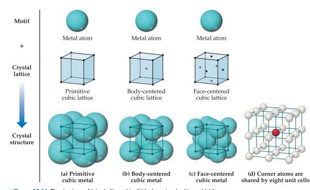
▲ Figure 12.11 The structures of (a) primitive cubic, (b) body-centered cubic, and (c) facecentered cubic metals. Each structure can be generated by the combination of a single-atom motif and the appropriate lattice. (d) Corner atoms (one shown in red) are shared among eight neighboring cubic unit cells.
