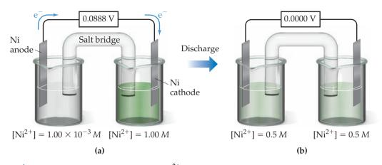
▲ Figure 20.14 Concentration cell based on Ni<sup>2+</sup>−Ni cell reaction. (a) Concentrations of Ni<sup>2+</sup> (*aq*) in the two half-cells are unequal, and the cell generates an electrical current. (b) The cell operates until [Ni<sup>2+</sup> (*aq*)] is the same in the two half-cells, at which point the cell has reached equilibrium and the emf goes to zero.
