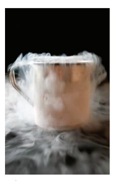
▲ Figure 10.11 Carbon dioxide gas flows downward because it is denser than air.
