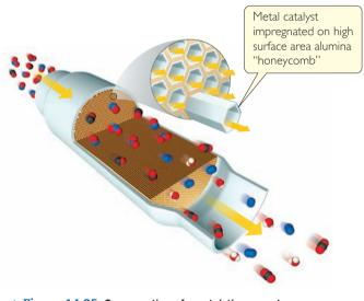
▲ Figure 14.25 Cross section of a catalytic converter.
