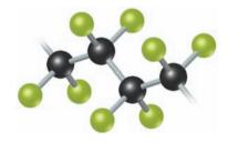
▲ Figure 22.9 Structure of Teflon<sup>®</sup>, a fluorocarbon polymer.
