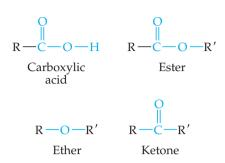
R, R', and R" represent hydrocarbon groups—for example, methyl (CH<sub>3</sub>) or phenyl ( $C_6H_5$ ).
