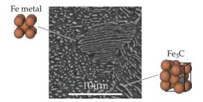
▲ Figure 12.16 Microscopic view of the structure of the heterogeneous alloy pearlite. The dark regions are body-centered cubic iron metal, and the lighter regions are cementite, Fe<sub>3</sub>C.
