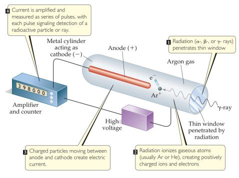
▲ Figure 21.9 Schematic drawing of a Geiger counter.
