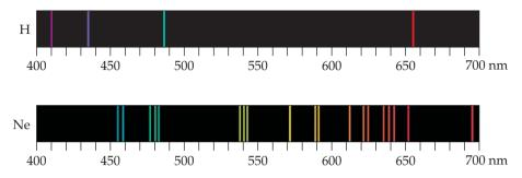
▲ Figure 6.11 Line spectra of hydrogen and neon. The colored lines occur at wavelengths present in the emission. The black regions are wavelengths for which no light is produced in the emission.
