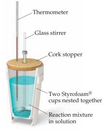
▲ Figure 5.17 Coffee-cup calorimeter. This simple apparatus is used to measure temperature changes of reactions at constant pressure. the water to the reaction (endothermic). In other words, by monitoring the temperature of the solution, we are seeing the flow of heat between the system (the reactants and products in the solution) and the surroundings (the water that forms the bulk of the solution).
