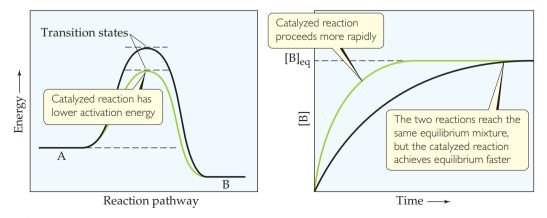
▲ Figure 15.14 An energy profile for the reaction A B (left), and the change in concentration of B as a function of time (right), with and without a catalyst. Green curves show the reaction with a catalyst; black curves show the reaction without a catalyst.
