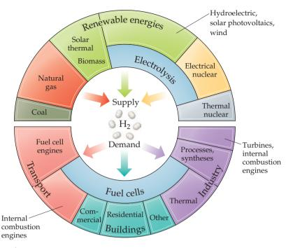
▲ Figure 22.4 The "hydrogen economy" would require hydrogen to be produced from various sources and would use hydrogen in energy-related applications.
