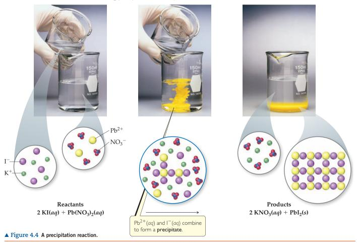
In Figure 4.4 the precipitate is lead iodide  $(PbI_2)$ , a compound that has a very low solubility in water:
