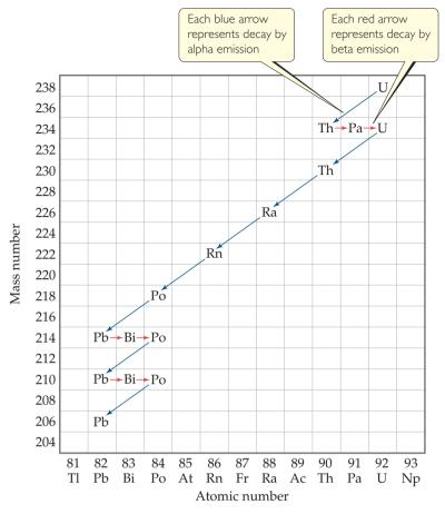
▲ Figure 21.3 Nuclear decay chain for uranium-238. The decay continues until the stable nucleus <sup>206</sup>Pb is formed.
